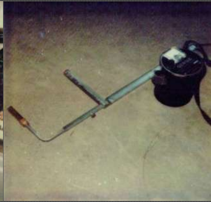
Liquid level gauge ^{60}\text{Co} : 20 MBq
